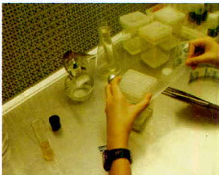
Seal the container with paraffin film.
