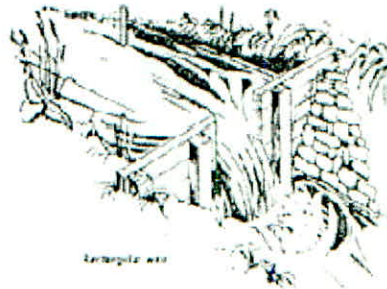
Fig. 2. Measuring stream flow with sharp-crested weirs
